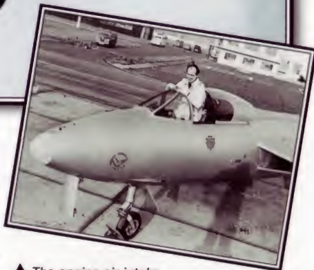
▲ The engine air intake proposed for the nose of the original design was moved to the wingroots on either side of the fuselage. Radar ranging equipment replaced it.
